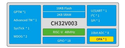
The muNico board provided by AtrivaTech utilizes the F4 P6 version of the CH32V003 which is fully compatible with existing opensource software development kits and specialized software CH32V003FUN by Charles Lohr and Arduino IDE plugin provided by WCH themselves.
